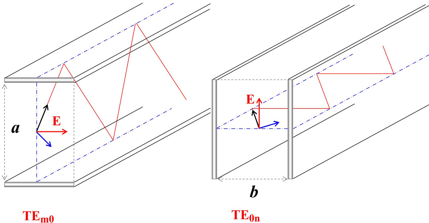
The **TE modes** of a parallel plate wave guide are preserved if perfectly conducting walls are added perpendicularly to the **electric field**.
