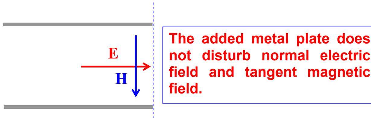
On the other hand, **TM modes** of a parallel plate wave guide disappear if perfectly conducting walls are added perpendicularly to the **magnetic field**.
