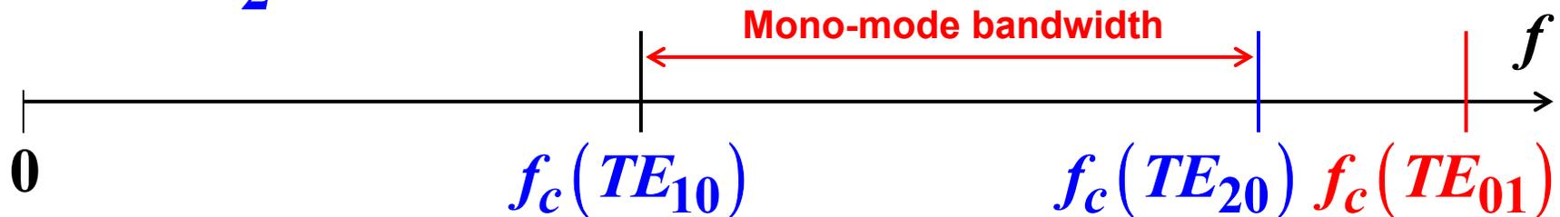
In practice, a **safety margin** of about **20%** is considered, so that the **useful bandwidth** is less than the maximum mono-mode bandwidth. This is necessary to make sure that the first mode ( $TE_{10}$ ) is well **above cut-off**, and the second mode ( $TE_{01}$  or  $TE_{20}$ ) is strongly **evanescent**.
