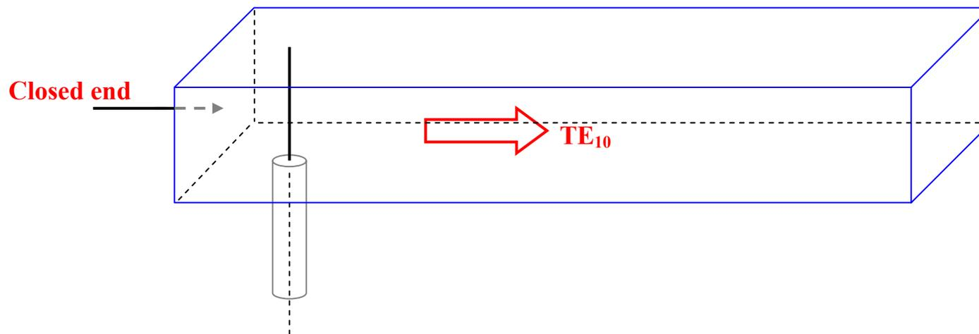
The **inner conductor** of the **coaxial cable** behaves like an **antenna** and it creates a **maximum electric field** in the middle of the cross-section.
