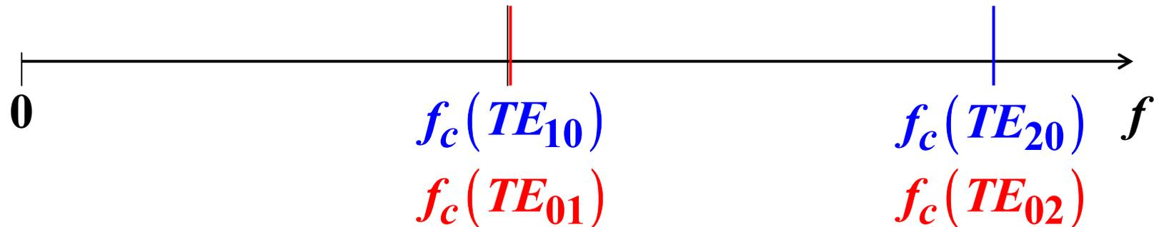
In the case of perfectly square wave guide,  $TE_{m0}$  and  $TE_{0n}$  modes with  $m=n$  are **degenerate** with the same cut-off frequency.
