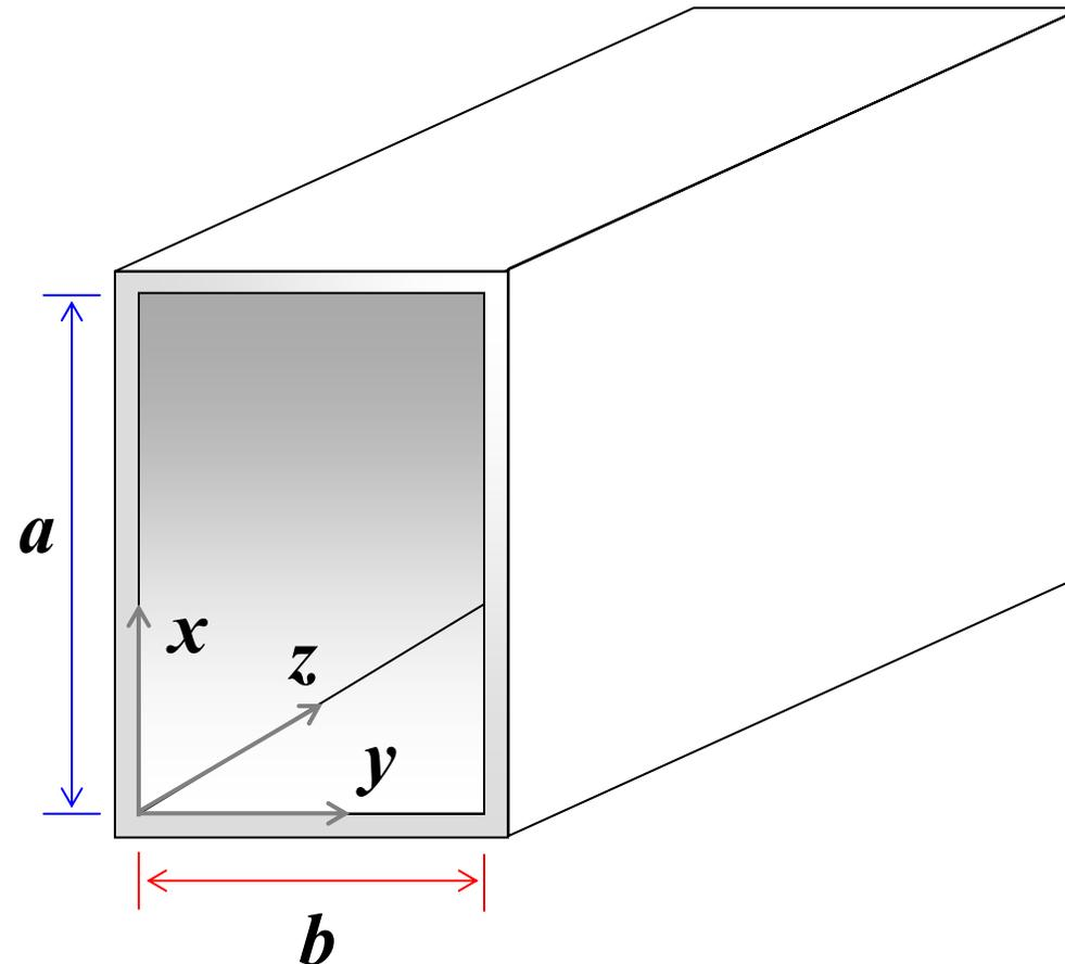
Assume **perfectly conducting** walls and **perfect dielectric** filling the wave guide.
